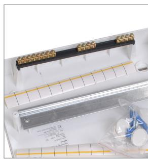
The special support for N and PE busbars can be easily removed and installed in both the upper and lower parts of the enclosure base. The support self-extinguishes at a temperature of 960°C.
