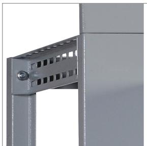
Use of flanges on vertical racks and vertical angles, preventing axial rotation of side ties, allows using half the number of fastening elements for assembly compared to the previous design.
