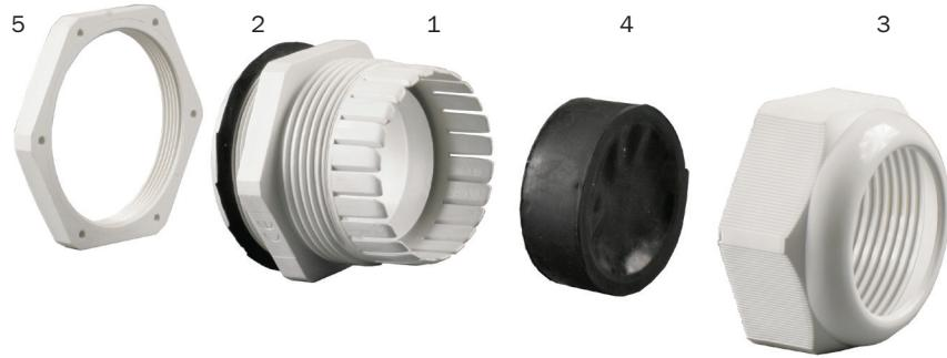
The gland consists of an enclosure (1), a seal (4), a packing nut (3), a gasket (2) and a fixing nut (5). The gasket and seal are made of neoprene.
