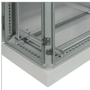
The cabinet can be equipped with a mounting panel that can be fixed at any required depth. The advantage is the possibility of installing the panel in the extreme position of the rear of the cabinet (flush with the frame), which allows optimal use of the usable space.
