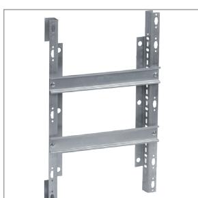
The removable mounting frame provides convenience and ease of assembly, the ability to mount outside the enclosure. DIN rails are installed with a pitch of 125 mm. For the convenience of cable routing, the distance between the rear wall and DIN rails has been increased.
