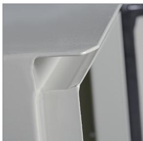
Protective visor and protective groove in IP54 enclosures – protection of electrical equipment from moisture penetration.
