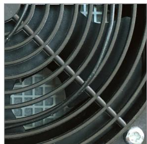
The direction of the cooling air can be easily changed by turning the fan over.
