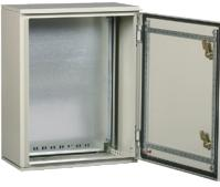
Metal enclosure with mounting panel-2-0<br>N1 IP65 GARANT   | Enclosure: 500×400×220<br>Panel: 394×340.<br>The total height of the panels<br>LG/LMA - 450    | 13         | YKM40-02-65 |
