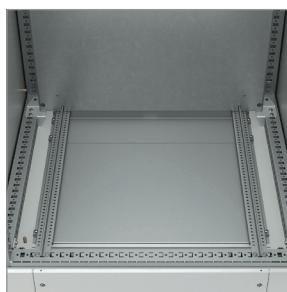
The bottom panel is made in the form of three movable plugs. It is possible to remove the bottom panel of the frame together with the plugs, which will allow you to obtain a cable gland with dimensions along the perimeter of the base of the cabinet.
