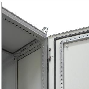
The prefabricated structure based on a frame made of closed-section profiles provides a high load capacity of the cabinet. On the mounting panel – 500 kg. On the door – 50 kg. Side/back panel – 50 kg. On the frame (on internal rails) – 1 600 kg.
