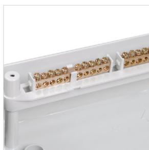
The removable N and PE busbar holder can be installed both at the top and at the bottom of the enclosure on special mounts. The N and PE tires themselves are installed on a removable holder by simply snapping into the seats.
