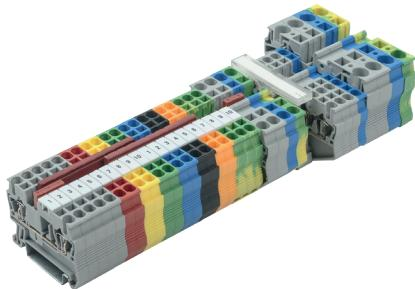
The spring-loaded type of conductor clamp provides fast assembly speed and secure hold under vibration loads. Double functional row of jumpers facilitates the task of potential distribution.
